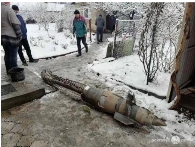
Forward end of the 9M54-series missile recovered in Pokrovsk. 10
