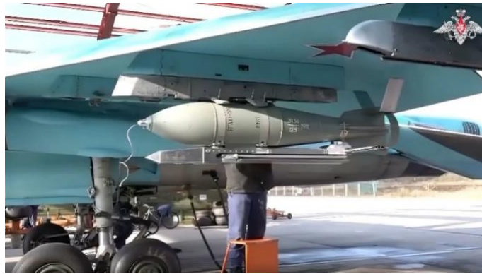
Figure 9: A UMPB glide bomb strapped on a Su-34 70
